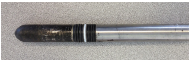
Damaged Gas Lift Valve
