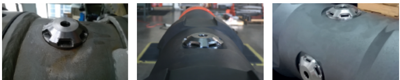
FloCheck Injection Valve installed in injection sub
