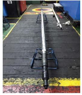
TAQA designed a slickline compatible Filtrex solution (2.5m in length) to have a standardised product to cover all customer wells in the campaign. The system provided the flexibility to be installed thru-tubing, beyond tight restirctions, whilst offering compliance to the damaged section once set.
