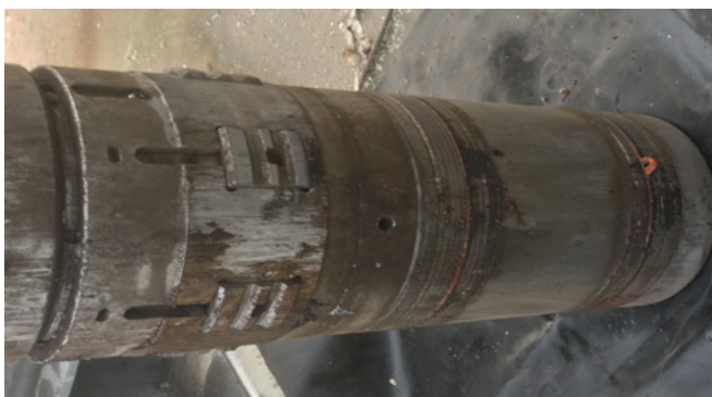
Injection sleeve retrieved from well with Encapsulated O-Rings still intact.
