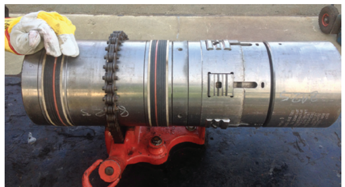
Injection sleeve and Encapsulated O-Rings cleaned after retrieval from the well.
